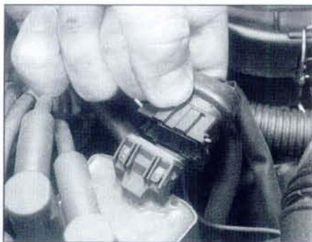
3.7 On models with a static (distributorless) ignition system, disconnect the wiring connector from the HT coil . . .
