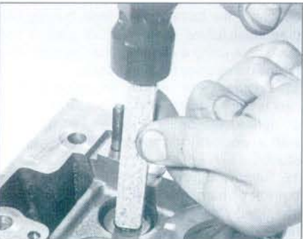
8.5 Remove the spring compressor, and tap the end of the valve to seat the collets in position
