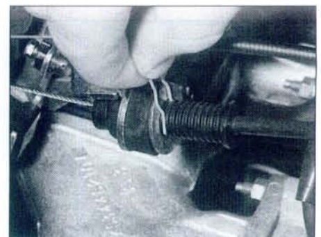
7.15 Adjusting the accelerator cable
