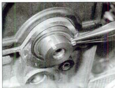
8.2 Removing the camshaft oil seal
