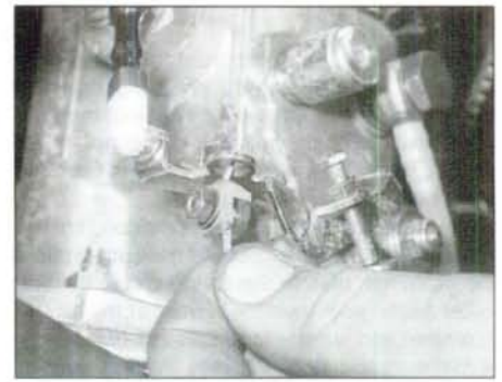
10.3 Slacken the clamp nut, and slide the end fitting off the fast idle cable
