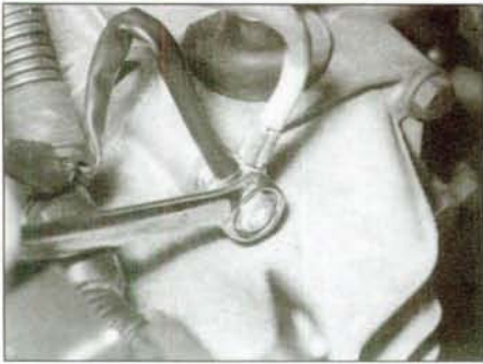
8.7 Undo the retaining nut, and release the earth straps from the top of the transmission housing
