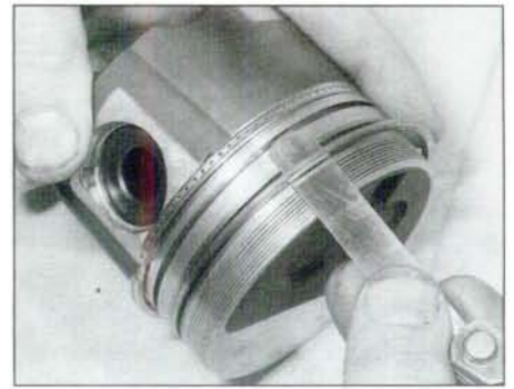
12.2 Removing a piston ring with the aid of a feeler gauge
