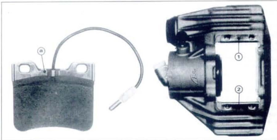
4.23 If fitting later-type pads with anti-rattle plate (a) to an earlier caliper, remove stainless plates (1) and (2)
