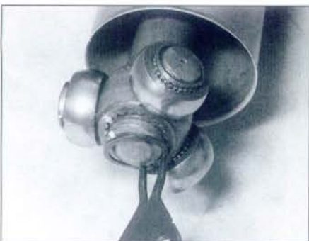
3.16 Removing the inner tripod joint securing circlip
