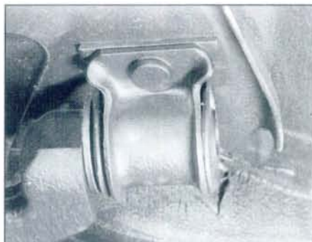
4.5b . . . that secure the suspension arm rear mounting
