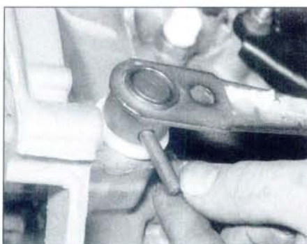
6.3b . . . tap out the retaining pin . . .
