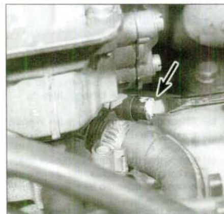
18.7a Mixture adjustment screw (arrowed) - Solex 32 PBISA carburettor (954 cc, 1124 cc and 1360 cc engines)
