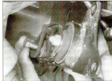
8.15b . . . then undo the bolt securing the mounting link to the body, and remove the mounting assembly from the vehicle
