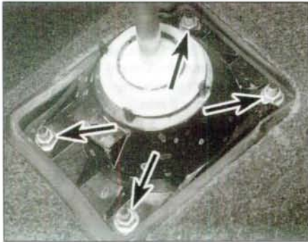
4.6a Gearchange lever retaining nuts (arrowed)
