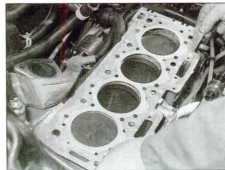
11.35b . . . and fit a new gasket
