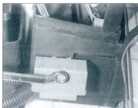
13.40b . . . then undo the retaining bolt, and remove the fuel injection relay unit
