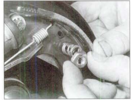
5.4b . . . to remove the outer hold-down spring cups, and remove the springs and pins
