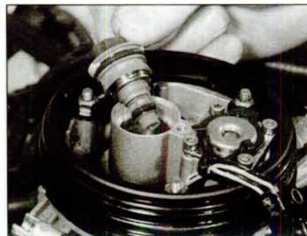
14.3b . . . then lift off the cap and withdraw the injector
