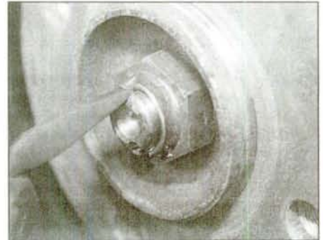
2.4 Relieve the retaining nut staking with a suitable cold chisel
