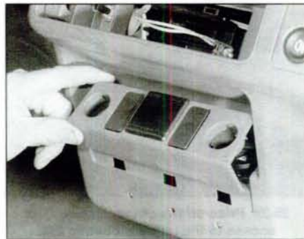
28.7 Removing the switch panel trim
