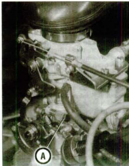
18.4b Idle speed adjustment screw (A) - early Weber 32 IBSH carburettor (954 cc engine)
