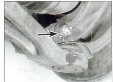
3.10 Hub carrier-to-lower arm clamp bolt (arrowed)
