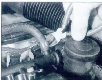
13.3 Where original crimped-type Citroën hose clips are fitted, cut and discard them
