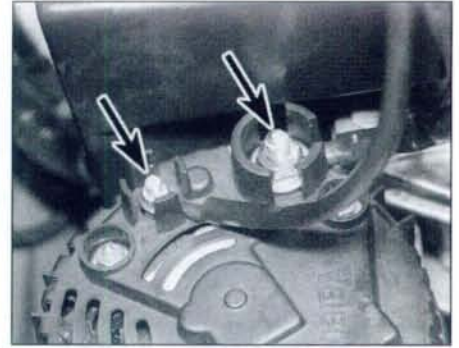
7.3 Undo the retaining nuts (arrowed) and disconnect the wiring from the rear of the alternator
