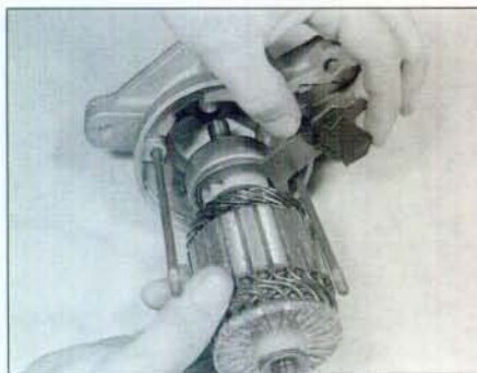
11.8 Withdrawing the armature from the drive end bracket
