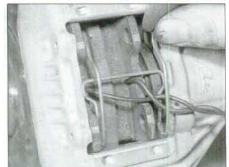
4.21 Removing the pad retaining spring
