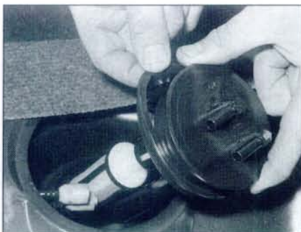
6.7 . . . then lift out the pick-up unit, and recover the rubber sealing ring
