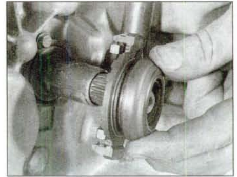
6.9 Install the release bearing, ensuring that its hooks are correctly engaged with the release fork
