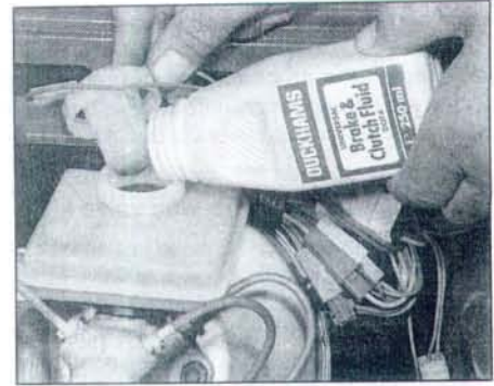
2.7 Topping-up the hydraulic fluid level in the reservoir
