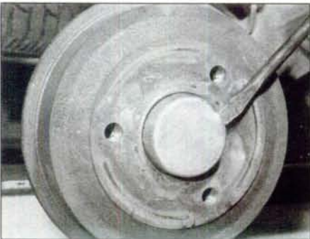
7.2a Carefully tap off the dust cap ...
