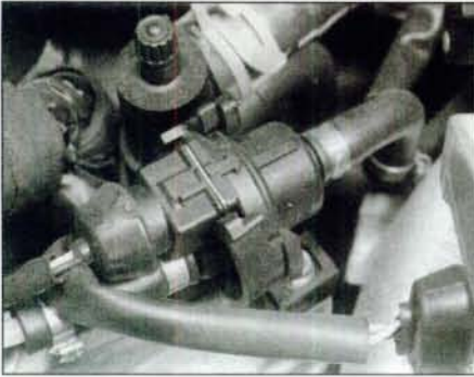
2.16 The purge valve(s) can be found in the right-hand rear corner of the engine compartment
