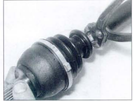
3.10 Securing a gaiter securing clip using side cutters
