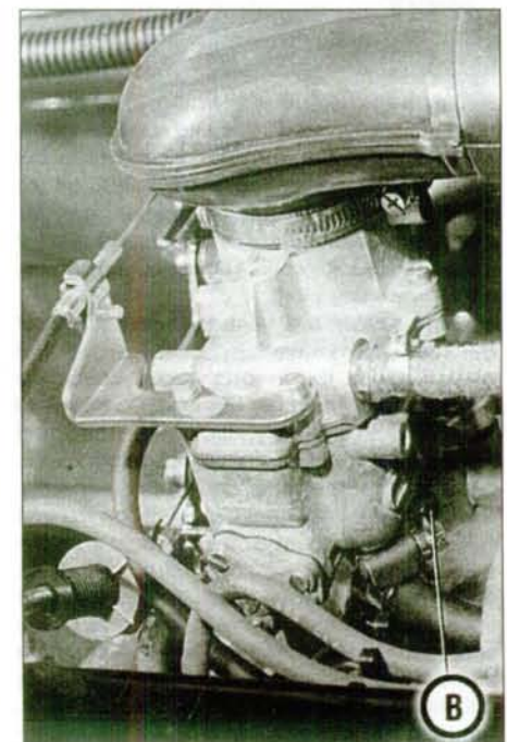
18.7b Mixture adjustment screw (B) - early Weber 32 IBSH carburettor (954 cc engine)
