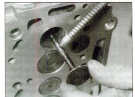
8.1 Lubricate the valve stems prior to refitting the valves
