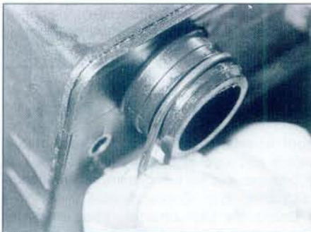
27.17b Check the air cleaner cover O-rings for signs of damage, and renew if necessary
