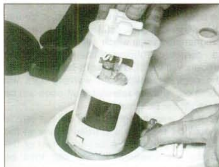
9.7a ... then lift out the fuel pump ...
