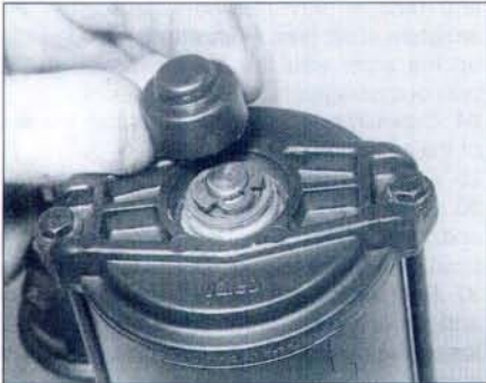
11.13 On the Valeo starter motor, remove the plastic cap from the end of the starter motor armature shaft ...
