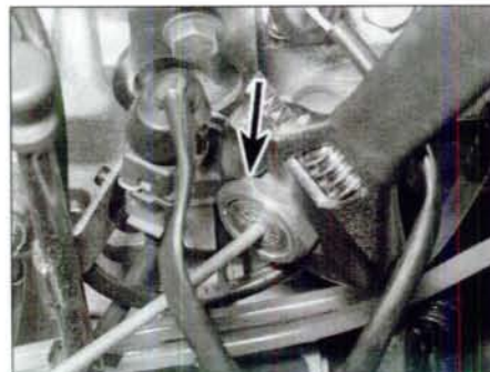
10.5a Unscrew the fast idle valve (arrowed) from the cylinder head . . .
