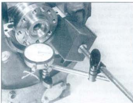
13.2 Checking crankshaft endfloat using a dial gauge
