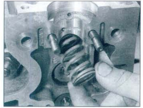
8.3a Refit the valve spring ...
