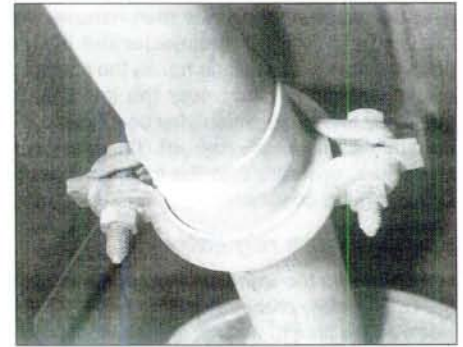
18.10 Typical exhaust system clamp
