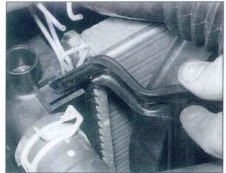
5.9b . . . and disengage the cooling fan shroud legs from the radiator brackets
