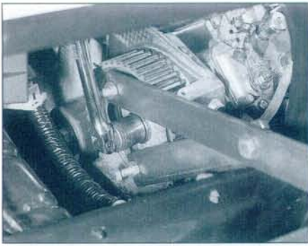
7.20 Using a home-made tool to hold the injection pump sprocket stationary whilst the retaining bolt is slacked - viewed through headlight aperture
