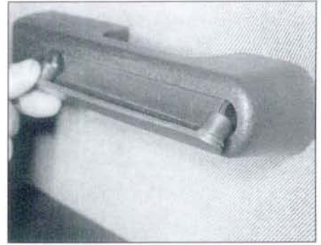
12.2b Removing the plastic cover for access to the armrest screws (later models)
