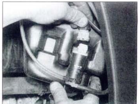
18.7 Disconnecting the wiring plug(s) and the hose(s)
