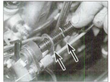
12.7b . . . then withdraw the outer cable from the mounting bracket, and recover the washer and spring clip (arrowed)
