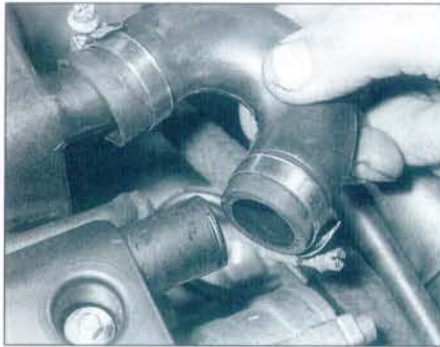
4.1 Slacken the retaining clip and disconnect the breather hose from the left-hand end of the cylinder head cover
