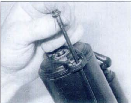
11.15a Remove the through-bolts ...
