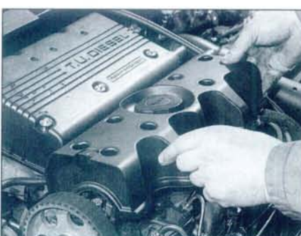
4.4 Lift the cover away from the engine, and recover the rubber seal
