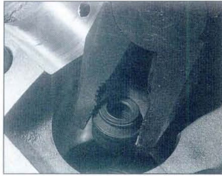
6.4b Remove the valve stem oil seal using a pair of pliers
