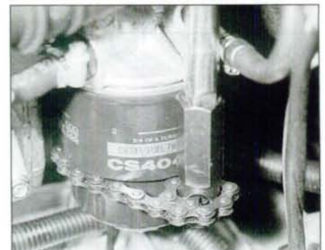
10.4 On Diesel models, if necessary, a chain wrench can be used to unscrew the fuel filter
