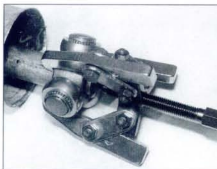
3.17a Using a three-legged puller to remove the inner tripod joint
