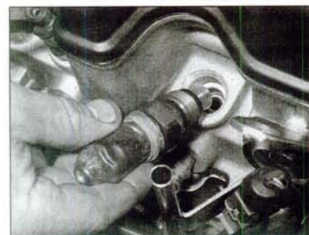
15.6 Unscrew the injector, and remove it from the cylinder head - note cover over the pipe opening, secured with an elastic band
