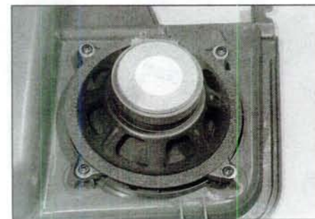
21.2b Speaker and mounting screws
