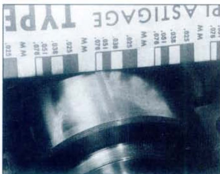
17.19 Measuring the width of the deformed Plastigage using the scale on the card provided
