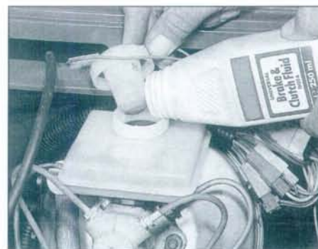
3.12 Topping-up the brake fluid level
