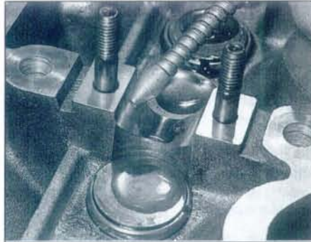
9.11 Thoroughly oil the camshaft bearing surfaces prior to installing the camshaft
