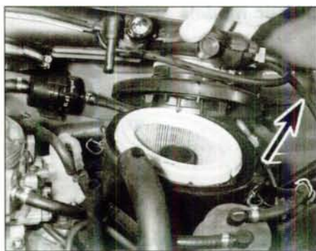
2.2b ... and remove the duct, disconnecting the air temperature control valve hose (arrowed)
