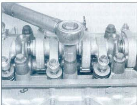
11.38b Working in the sequence shown, tighten the head bolts first to the Stage 1 torque setting ...
