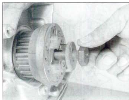
7.11a Remove the crankshaft sprocket retaining bolt . . .
