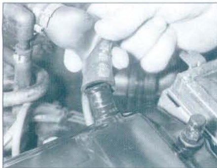
4.3 Disconnect the breather hose from the cylinder head cover . . .
