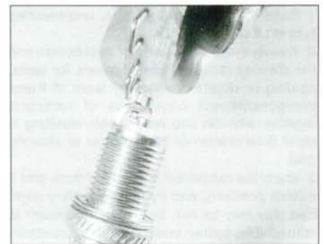
14.9c Adjusting the gap using a special adjusting tool
