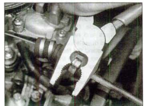
9.11 Cutting the original crimped-type hose clip from the choke cable rubber collar
