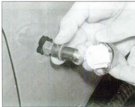
5.18 Disconnecting the bulbholder from the side repeater lens
