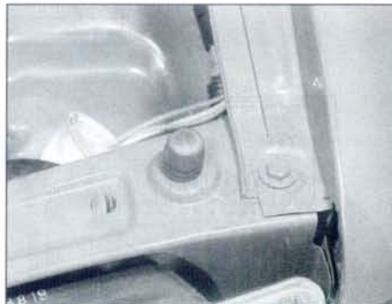
8.8 Adjust the rubber buffers up or down to align the front of the bonnet
