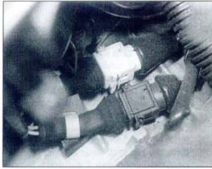
2.6b Trace the lambda sensor wiring back to the top of the transmission, then disconnect the connectors
