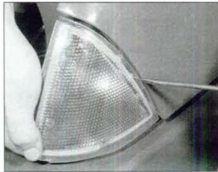
7.6a Release the tab using a thin-bladed screwdriver . . .
