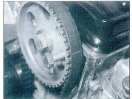
3.5 . . . then insert a 10 mm bolt through the camshaft sprocket timing hole, and locate it in the cylinder head
