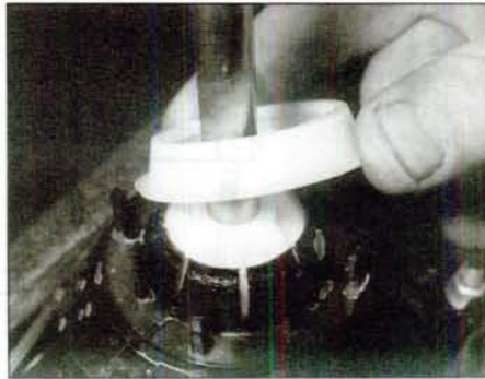
4.6b The gearchange lever can be separated from its baseplate once its retaining ring has been unclipped
