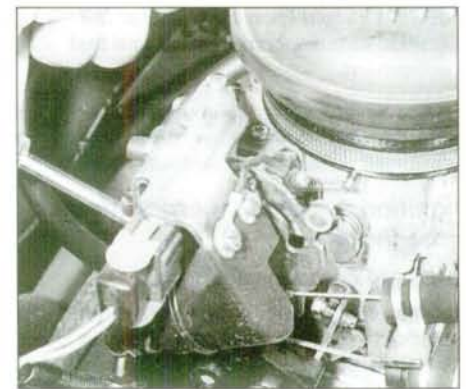
18.4e Adjusting the Idle speed - Solex 32-34 Z2 PSA carburettor (1360 cc engine)
