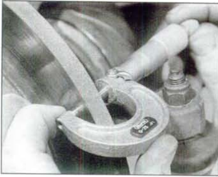
6.3 Using a micrometer to measure disc thickness
