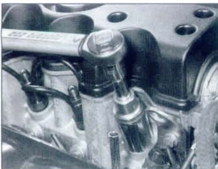
16.3 Slacken the retaining clip, and disconnect the air intake duct from the left
