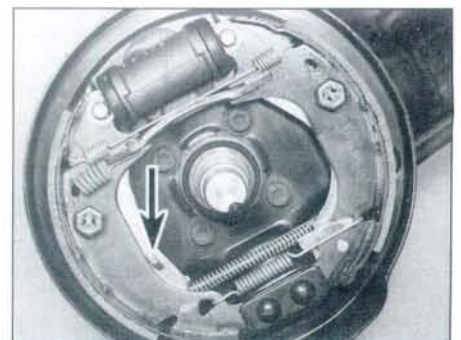
7.14 Ensure that the handbrake lever stop-peg (arrowed) is positioned against the edge of the shoe web
