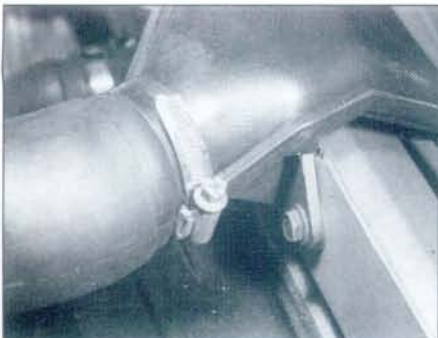
3.4 Air intake ducting bolted to crossmember (certain models only)
