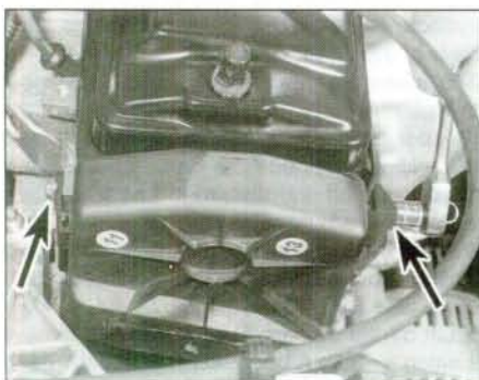
5.1a Undo the two retaining bolts (arrowed) . . .
