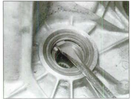
5.4 Use a large flat-bladed screwdriver to prise the driveshaft oil seal out of position
