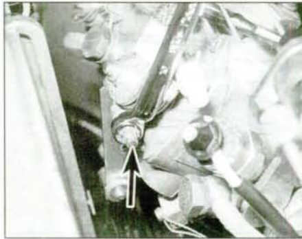
19.9 . . . then slacken the locknut and turn the screw (arrowed) to set the anti-stall speed
