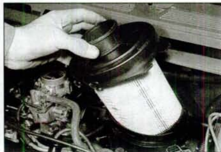
27.3 Removing the air cleaner cover - type with integral element
