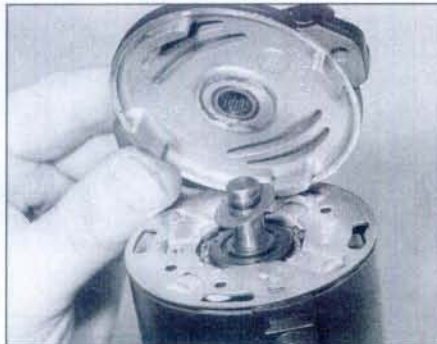
11.15b ... then withdraw the end cover, and recover the shim (arrowed)
