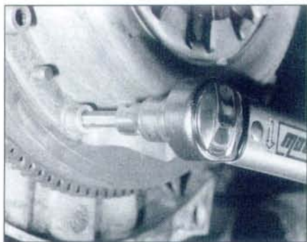
5.17 Once the friction plate is centralised, tighten the pressure plate retaining bolts to the specified torque
