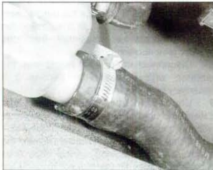
3.8 Radiator bottom hose connection
