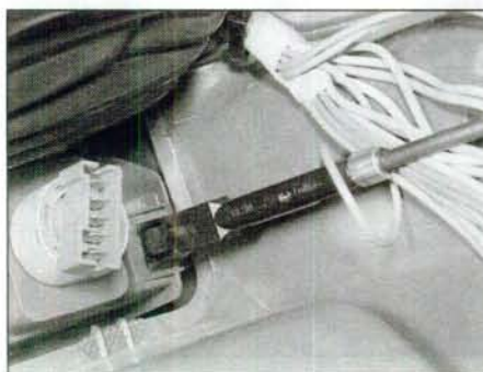
9.5a Choke cable attachment to fascia panel, viewed from inside
