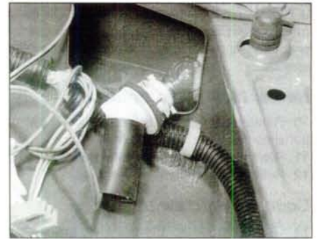
5.13 Front indicator light bulb and holder removal
