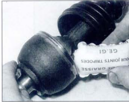
3.8 Pack the joint with the grease supplied in the repair kit
