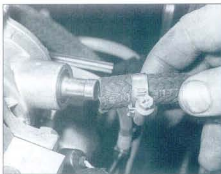
11.8 Slacken the retaining clip, and disconnect the hose from the braking system vacuum pump
