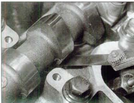
10.5 Measuring a valve clearance using a feeler gauge
