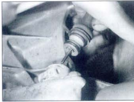
7.2b . . . then disconnect the speedometer cable from its drive
