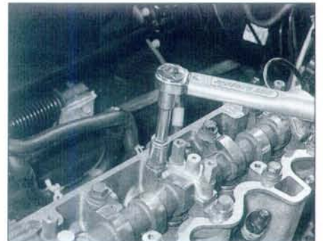
11.38b Tightening the head bolts with the torque wrench ...
