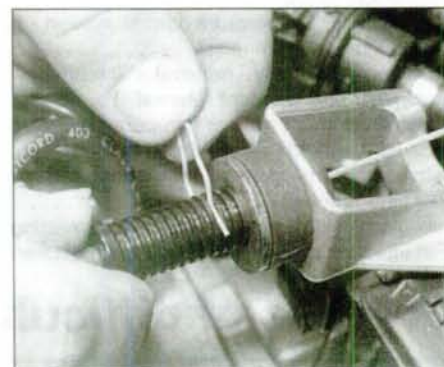
4.3 Adjust the accelerator cable as described in text
