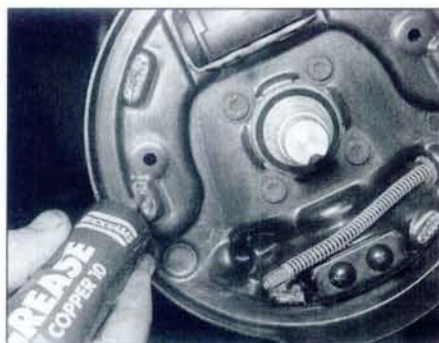
5.16 Apply brake grease to the shoe contact areas
