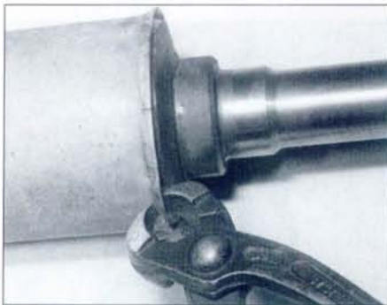
3.13 Peeling back the lip of the joint outer member cover
