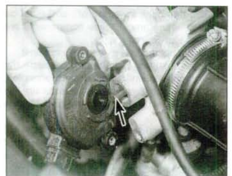
13.14 On refitting, ensure that the potentiometer is correctly engaged with the throttle valve spindle (arrowed)
