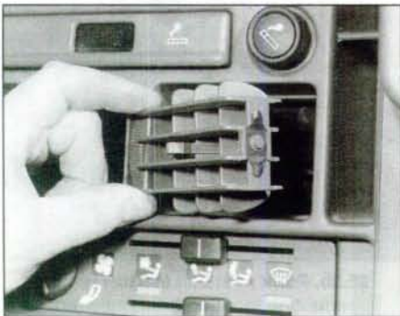
28.3 Removing a ventilation grille from the facia
