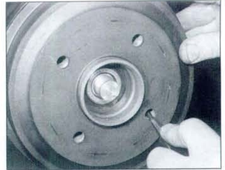
7.7a Using a screwdriver to release the shoe adjuster mechanism and retract the shoes (left-hand side of the car)
