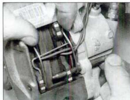
4.20d . . . and lower pins - ATE caliper
