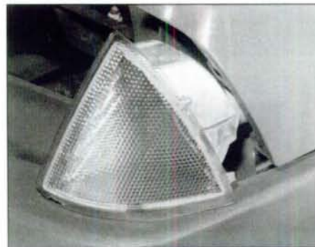
7.6c Front direction indicator, showing location pegs and slots in wing
