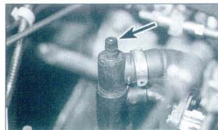
33.4b Bleed screw location (arrowed) in the heater return hose on a later 1124 cc (H1A engine) carburettor model
