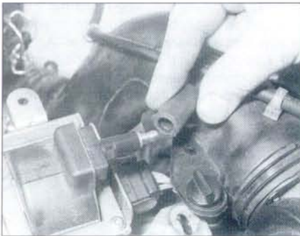
3.4a . . . then disconnect the HT lead . . .
