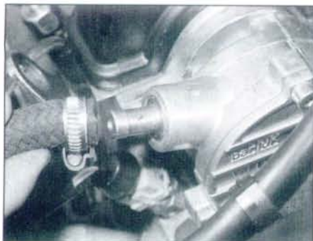
22.2 Disconnecting the vacuum hose from the brake vacuum pump - Diesel engine model
