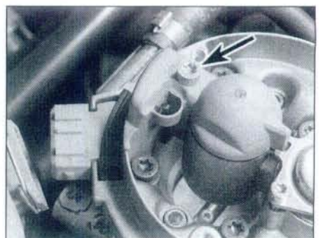
14.20 Disconnecting the injector wiring connector. Injector retaining screw is arrowed
