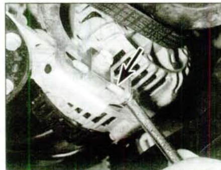
21.8a Loosen the alternator mounting bolts, then slacken the adjuster bolt (arrowed) . . .
