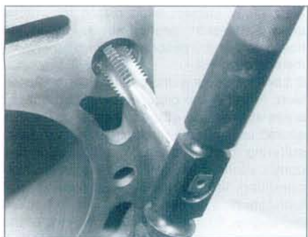
11.8 Cleaning a cylinder block threaded hole using a suitable tap
