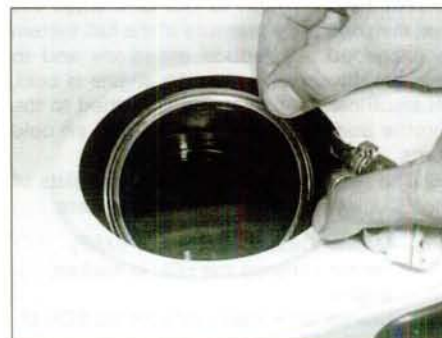
9.7b ... and recover the rubber sealing ring
