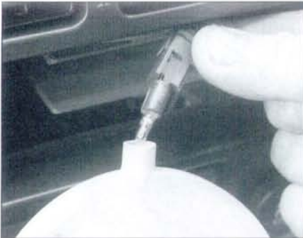
6.11 Removing the heater control panel illumination bulb
