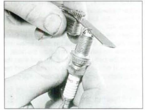
14.9b Measuring the spark plug gap with a feeler blade
