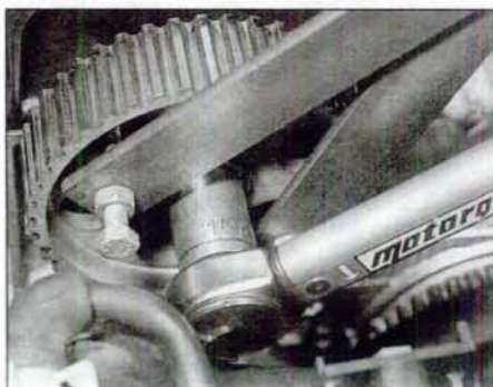
7.31 Tighten the camshaft sprocket retaining bolt to the specified torque setting
