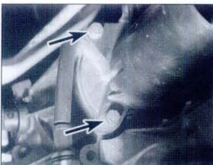
10.5a Undo the starter motor retaining bolts (rear two arrowed) . . .
