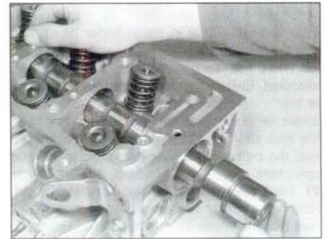
10.9b . . . and slide out the camshaft
