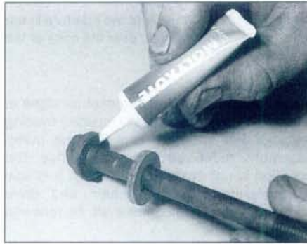
11.37a Apply a smear of the specified grease to the underside of the heads ...
