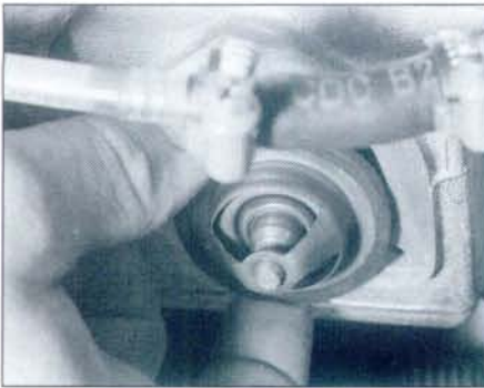
4.6 Lift the thermostat from the housing (Diesel model shown)
