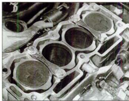
11.26 The cylinder liners must be clamped in position before the crankshaft is rotated
