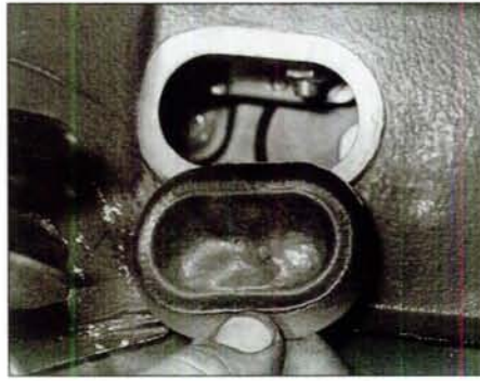
5.3a Remove the rubber plug from the right-hand wing valance ...
