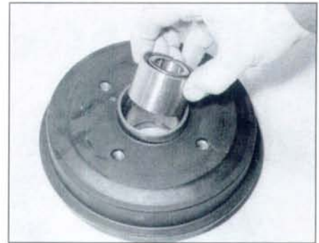
7.9a Locate the bearing in the hub ...
