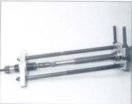
5.3 Using a long-reach bearing puller to remove the intermediate bearing from the right-hand driveshaft
