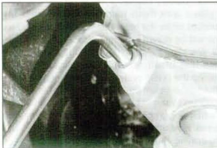
30.2 Using the square-section wrench to unscrew the transmission filler/level plug
