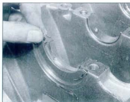
17.26 Refitting a crankshaft thrustwasher - aluminium block engines
