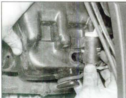
18.10 Removing a washer fluid pump
