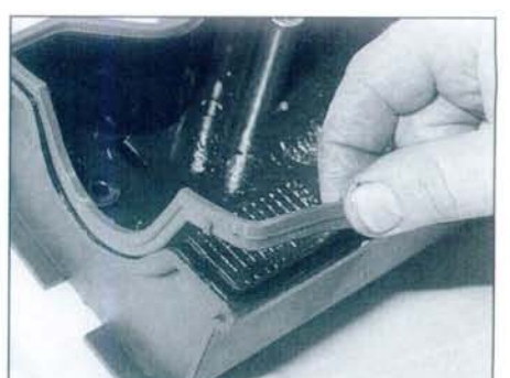
4.6 Ensure the new rubber seal is correctly located in the cover groove prior to refitting
