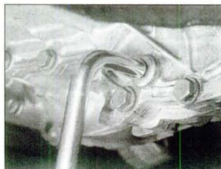
2.4 Using the special square-section wrench to unscrew the transmission drain plug
