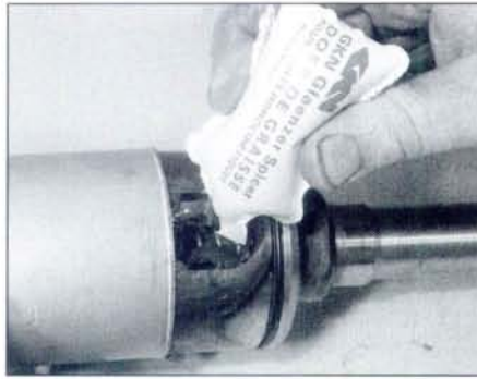
3.26b . . . then apply the remainder of the grease . . .
