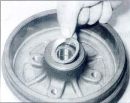
7.11a Fit the new oil seal thrust cup ...
