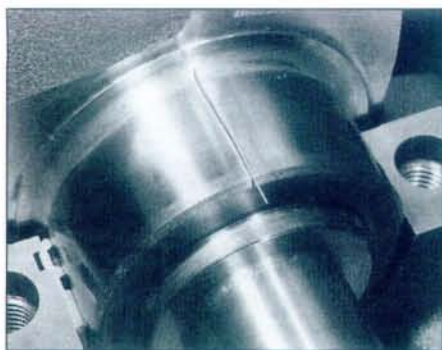
17.16 Plastigage in place on a crankshaft main bearing journal
