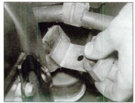
17.4c ... and recover the buffer plate from the mounting stud
