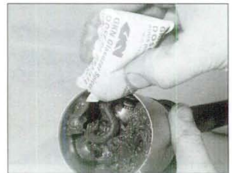
3.24 Pack the joint and gaiter/cover with grease
