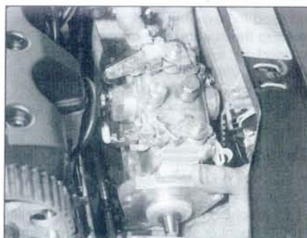
12.15b . . . and remove the injection pump from the engine
