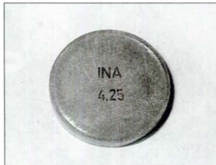
10.10a Shim thickness is stamped on the bottom face of the shim . . .
