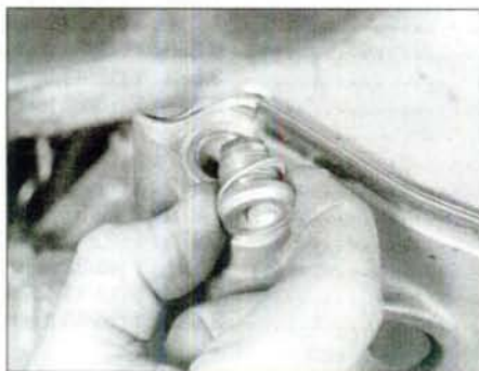
2.3 Unscrew the filler/level plug from the transmission, and recover the sealing washer
