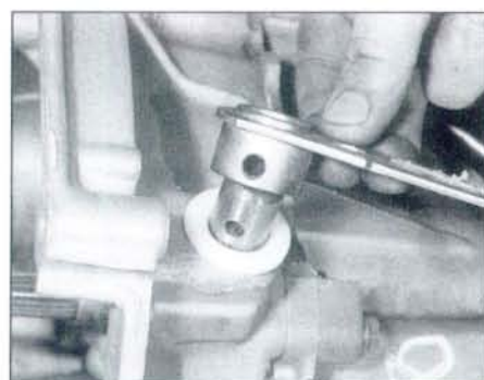
6.3c . . . then remove the release lever from the top of the release fork shaft
