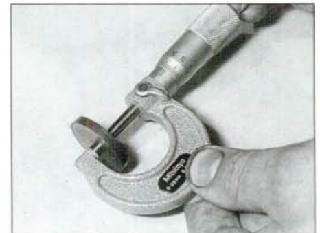
10.10b . . . however shims should be measured to determine their true thickness
