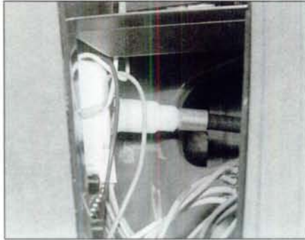
14.3 Speedometer cable-to-instrument panel connection viewed through the fusebox aperture - models up to July 1991
