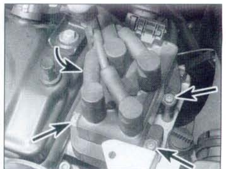
3.9 . . . then disconnect the HT leads from the coil. Undo the four retaining screws (arrowed) and remove the coil
