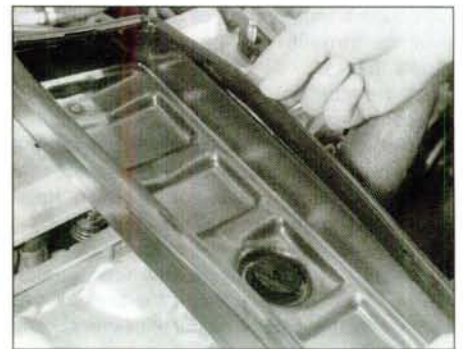
4.8 On refitting, ensure that the rubber seal is correctly located on the cylinder head cover
