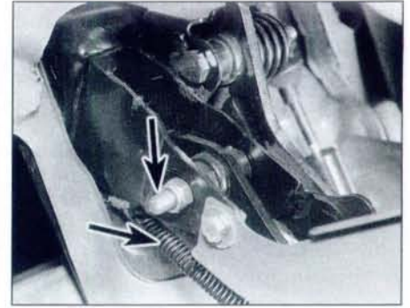
4.3 Pedal mounting assembly on right-hand drive models, showing pivot bolt and clutch pedal return spring (arrowed)
