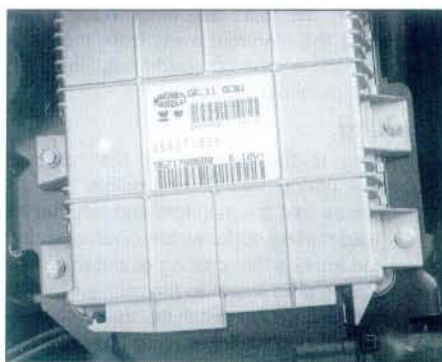
15.27 Magneti Marelli electronic control unit (ECU)
