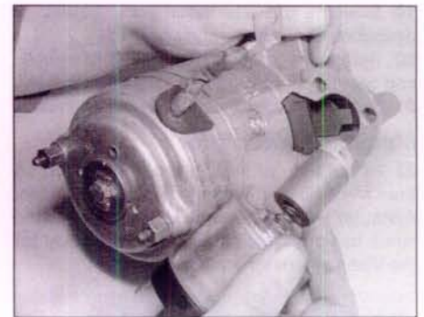
11.3 Removing the solenoid from the drive end bracket
