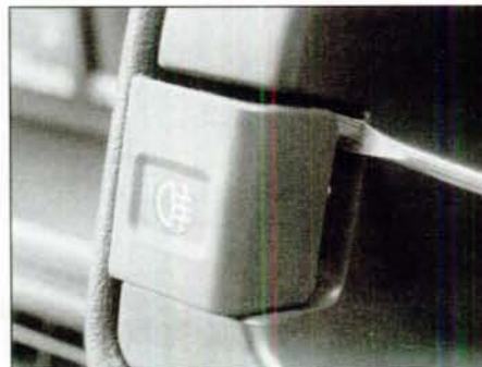
4.7a Use a screwdriver to prise the switch from the fascia
