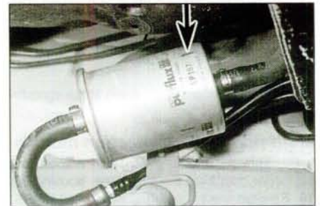
31.4 Release the strap and disconnect the hoses to remove the fuel filter. Note the direction of the arrow on the filter body (arrowed)
