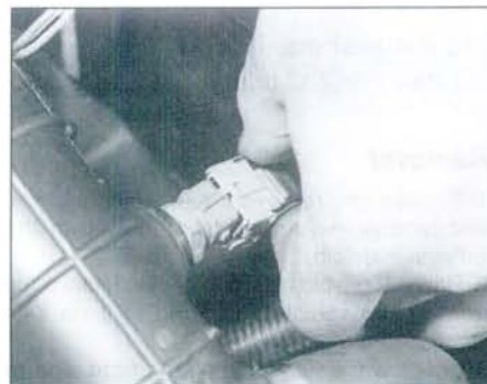
13.31 Disconnecting the wiring connector from the intake air temperature sensor
