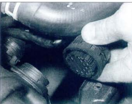
4.30a Disconnecting the main engine/transmission wiring harness connector . . .
