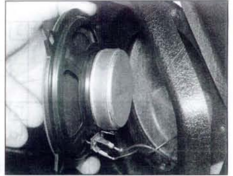
21.3c . . . and withdraw the speaker in order to disconnect the wiring
