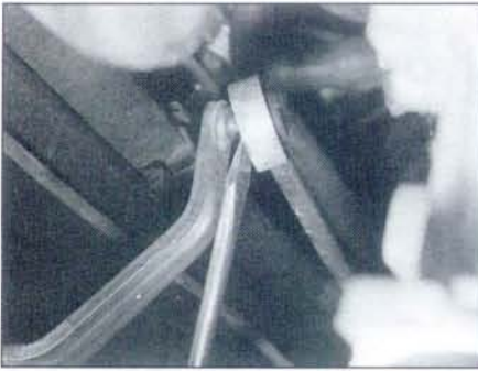
3.5 Carefully lever the link rods off their balljoints, using a large flat-bladed screwdriver
