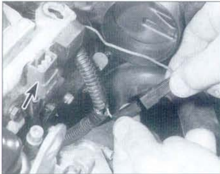
3.3 On models with a distributor, disconnect the capacitor wiring connector, and release the TDC sensor connector (arrowed) . . .
