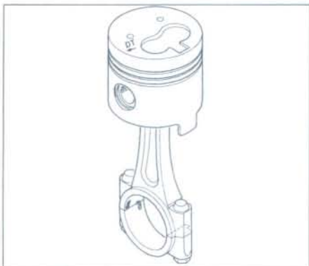
12.18 The cloverleaf recess in the crown must face the opposite way to the bearing shell cut-outs in the connecting rod
