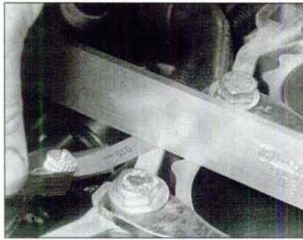
11.24 Checking cylinder liner protrusion - aluminium block engine
